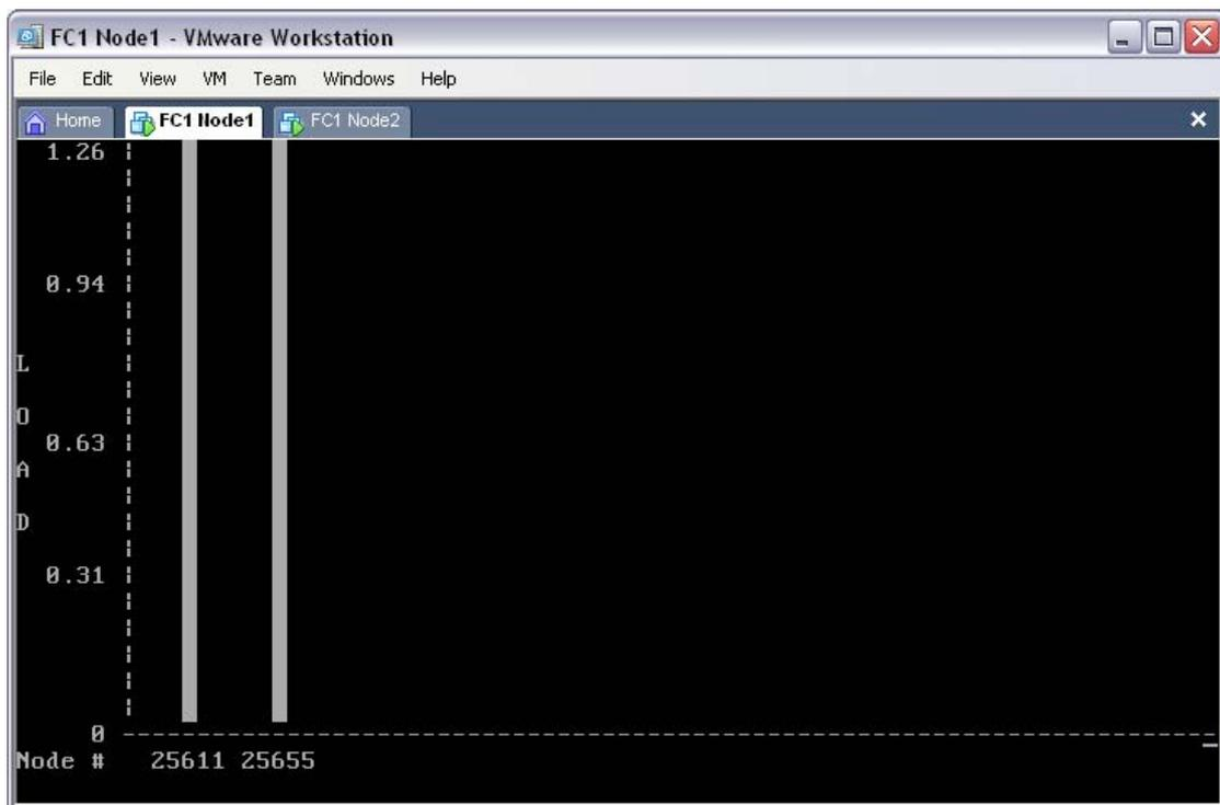
To see the load of each node in the cluster, from any node in the cluster, run the command “mosmon” – try this now, staying on the first node. Shown in this screen shot, the first node believes that both nodes are evenly distributing the load – indicating that there are two “omtest.sh” script instances on each node.
